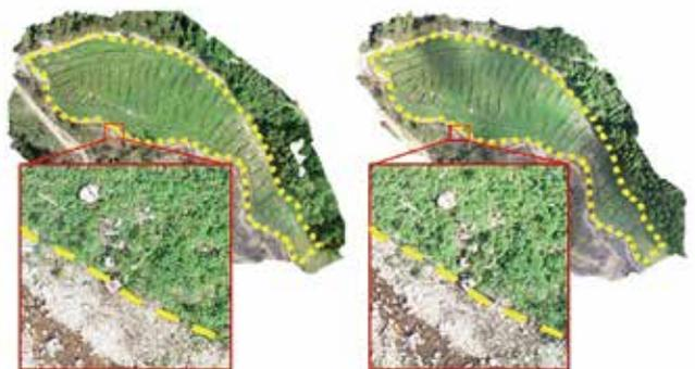
図2：飛行高度40m(左)と140m(右)の拡大比較
